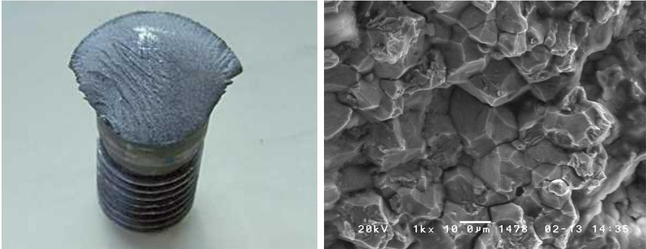
Intergranular cracking occurs when cracks form and grow along weakened grain boundaries in a metal. In the case of hydrogen embrittlement, the hydrogen bubbles at the [grain boundaries](#) weaken the metal.
