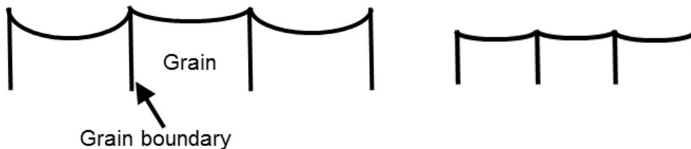
These figures show two samples of a sheet metal component. One component had small grains throughout. The other had large grains at the surface. The component with the large grains at the surface exhibited orange peel.
