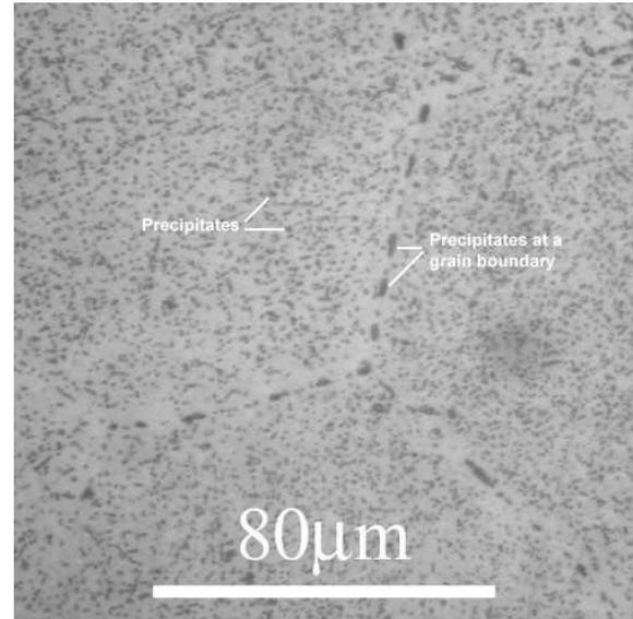
Only certain alloys can be precipitation strengthened. The 2xxx, 6xxx, and 7xxx alloys can be precipitation strengthened through the formation of Al-Cu (2xxx), Mg-Si (6xxx), and Al-Zn-Mg-(Cu) (7xxx) precipitates. The 1xxx, 3xxx, 4xxx, and 5xxx alloys cannot be precipitation strengthened.
