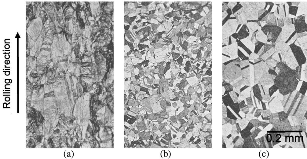
The cold-rolled sample had a yield strength of 80 ksi (550 MPa). The sample that was annealed at 1022 °F (550 °C) for 1 hour had yield strength of 11 ksi (75 MPa). Many small grains are present in this sample. The sample that was annealed at 1202 °F (650 °C) for 1 hour had yield strength of 9 ksi (60 MPa). Fewer, large grains were present in this sample compared to the sample in Figure (b).
