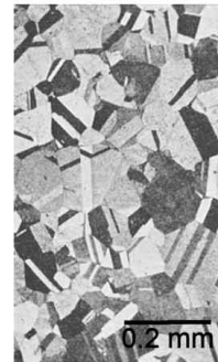
C 50% reduction 1202 °F (650 °C) anneal 9 ksi yield strength
